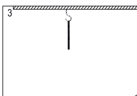
3. Drill 1x expanded screw hole and install it, and hang the chain as Fig.3.
